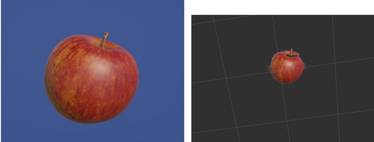
Fig. 1. Demonstration of the point cloud generation pipeline, a comparison of the raw left camera image and the corresponding generated point cloud.
